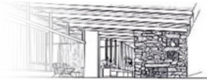
Looking from living room to entrance hall. Roof construction of Western Red Cedar planking and glued-laminated fir joists makes the interesting sloping ceiling. Wall on right is Douglas Fir Plywood. Hanging box, which is made of knotty Western Red Cedar, is suspended from ceiling.
